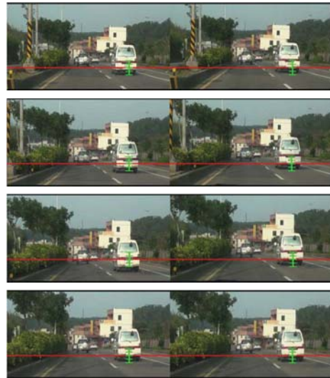
Fig. 4. Example for video stabilization. Left parts are original four consecutive frames during oscillation. Right parts are stabilized results.
